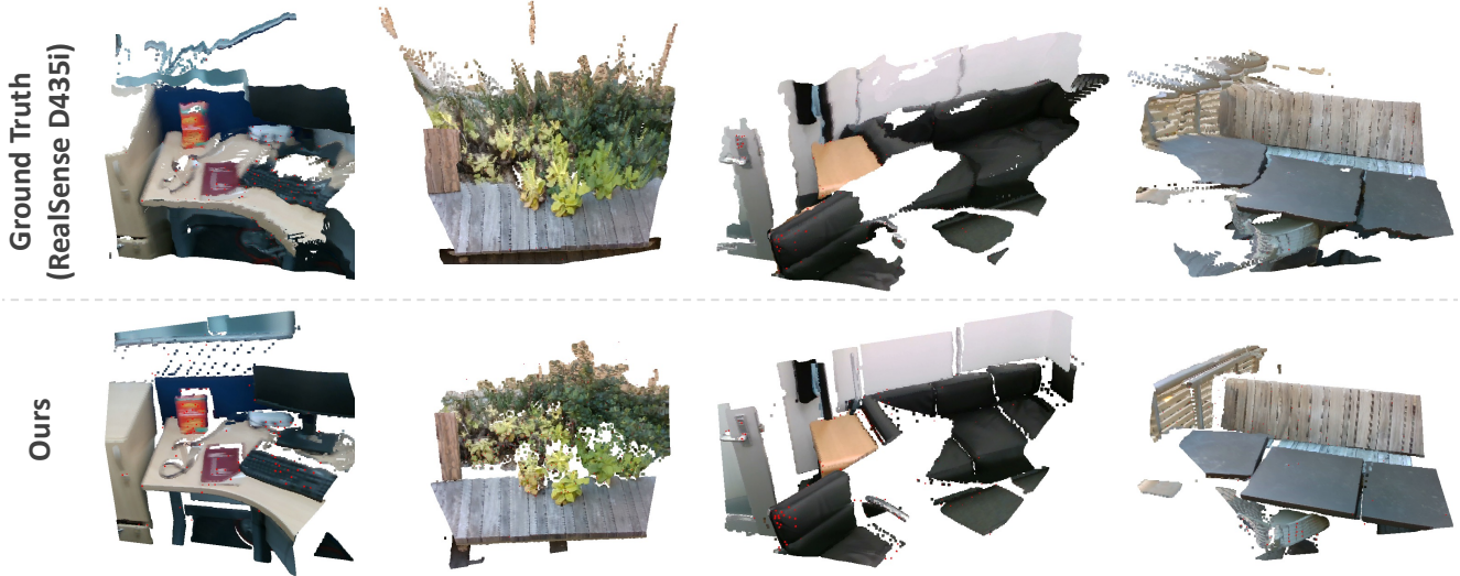
Figure 3. Depth Completion on VOID. We visualise the coloured unprojections of ground truth depth maps provided by a sensor (top row) and the geometry estimated by our method (bottom row). Sparse depth input points are visualised as red dots (electronic zoom-in recommended). Qualitatively, we achieve sharper geometry estimates than from a commodity depth sensor.
