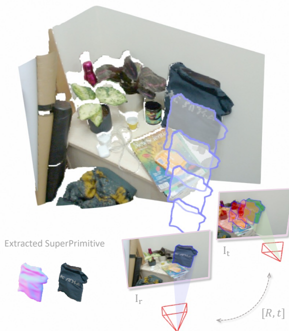
Figure 1. Multi-View Geometry with SuperPrimitives. SuperPrimitives are extracted from an input frame by dividing it into image segments equipped with estimated surface normal directions (bottom-left). Each SuperPrimitive induces a dense reconstruction within the corresponding image segment up to a a priori unknown scale. Different possible reconstructions are shown in light blue. The scales are then jointly optimised together with a relative camera pose to fit multi-view photometric constraints (visualised in green and red). The resulting dense reconstruction of the reference frame is shown in the top.
